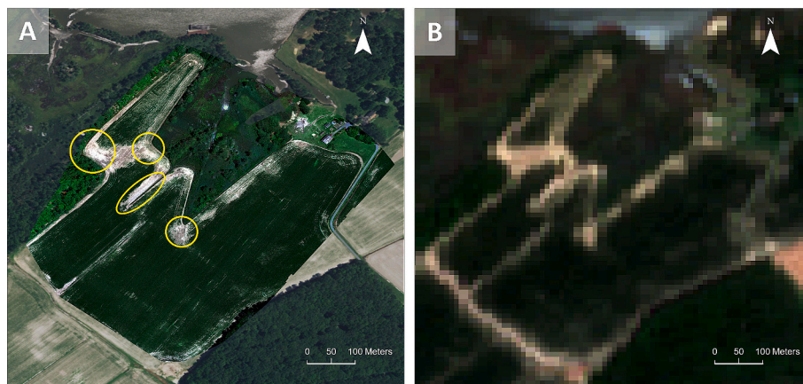
Fig. 3. True color images revealing saltwater intrusion effects on farmland: (A) High-resolution UAV image of the farmland (60 cm resolution) overlaid on NAIP imagery in the background (1 m resolution) with yellow circles highlighting locations of salt patch; (B) Sentinel-2 true color image (10 m resolution). (For interpretation of the references to color in this figure legend, the reader is referred to the web version of this article.)
