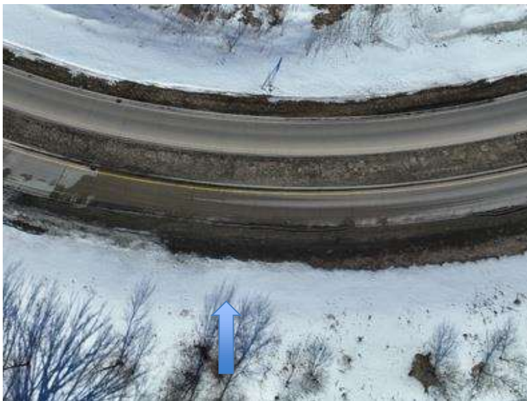
Figure 17. Super Elevated Surfaces Known for Meltwater Sprawl
