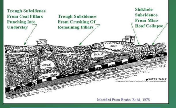
Subsidence: Any surface expression of AML-related subsidence which damages property and poses danger to human safety and health. These may be tension cracks, troughs, shearing faults, or caving caused by AML-related underground mine voids.
