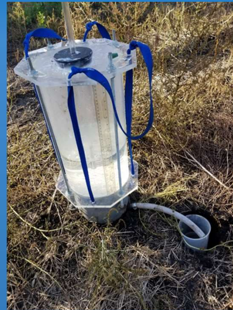
Infiltrometer to measure runoff
