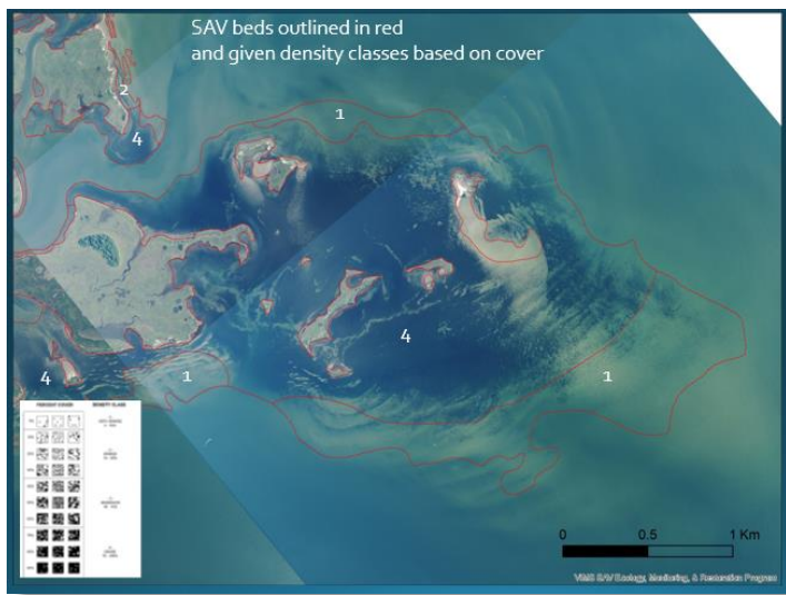
Figure 2. SAV polygon with assigned density classes based on classification protocols and professional judgement of percent cover. Cover classes range from 1 to 4: 1 = <10% SAV (Very sparse); 2 = 10% - 40% SAV (Sparse); 3 = 40% - 70% SAV (Moderate); 4 = 70% - 100% cover (Dense).
