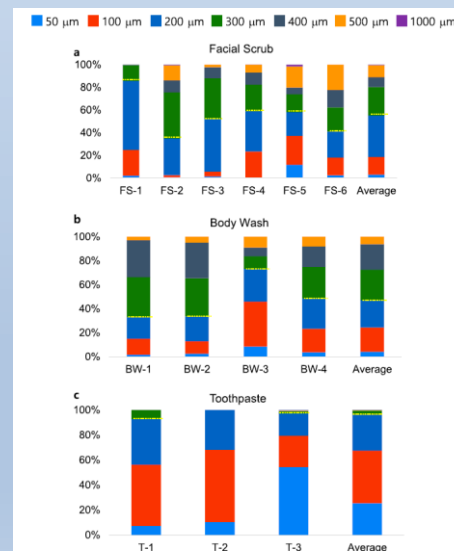
Fig. 1 Polyethylene microplastic mass size distribution by for a facial scrubs, b body wash and c toothpaste. Dotted yellow lines indicate the division between smaller (<300 \mu\text{m} ) and larger (>300 \mu\text{m} ) size classes
