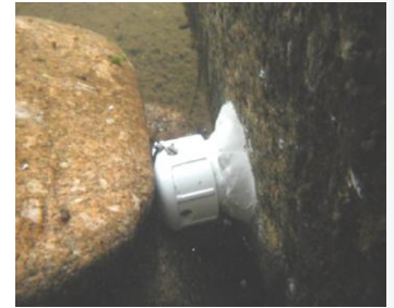
Underwater epoxy method
