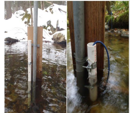
Vented vs. non-vented transducers
