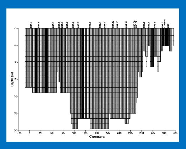
Elevation view of grid along a transect from the mouth of the bay (km 0) to the head of tide (≈ km 320). Note that variations in depth are represented by variations in the number of cells in the vertical dimension.
