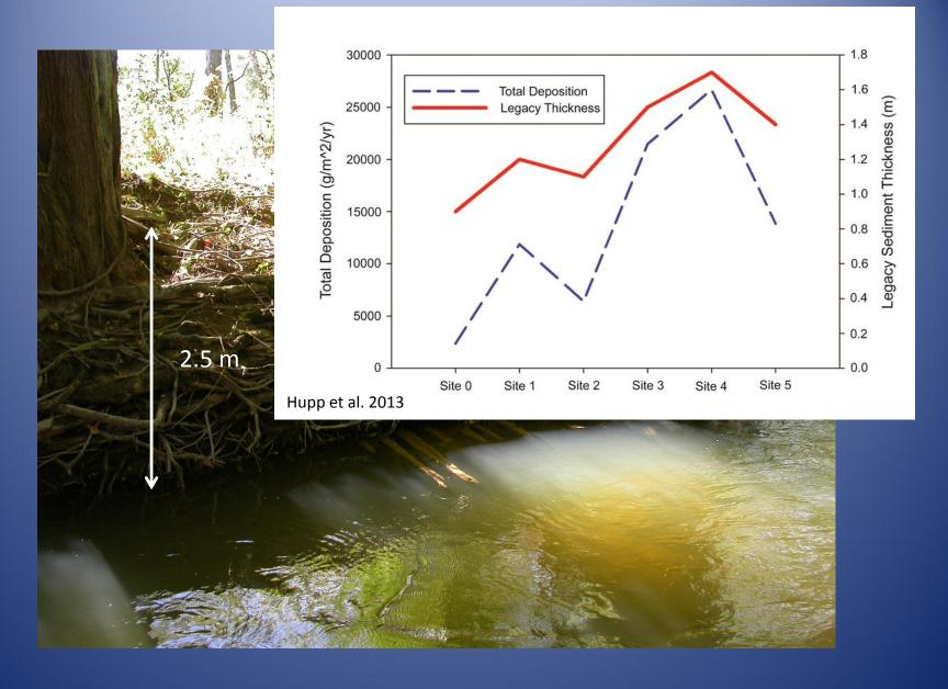
Difficult Run floodplain stores on average 132 cubic meters of sediment per meter of reach length.
