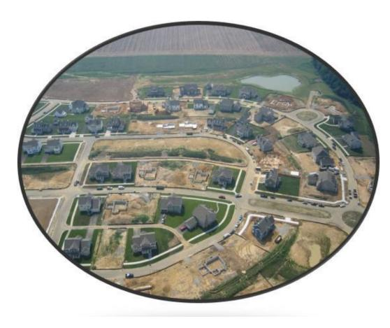
Construction process involves initial clearing and grading, earth-moving, installation of streets and storm drains, building construction and finally, the final stabilization of the site.
