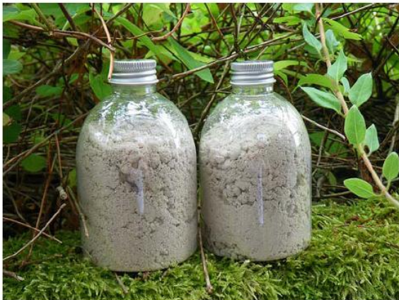
Figure 2-15 Struvite Produced from Urine at GTZ Headquarters (M. Winker, 2010). Reprinted with permission from GTZ.
